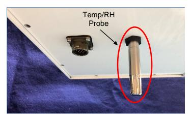
The solid state capacitive relative humidity sensor is easily replaced in the field. Simply: unscrew the cap on the TEMP/RH probe. Pull out the old INTERCAP element. Insert the new element. Screw the cap back on. Finished.
